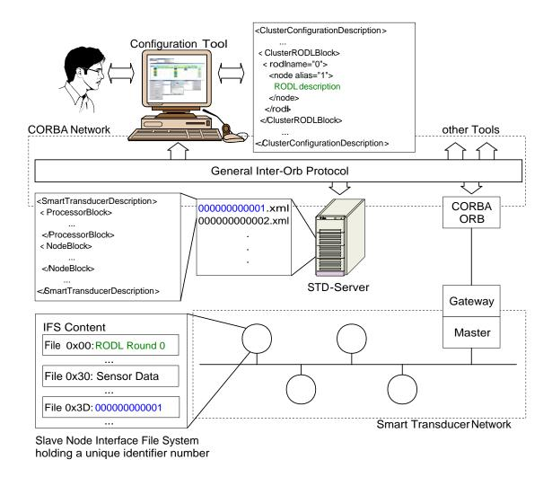
Figure 3: Configuration and management with remote tools for TTP/A networks
