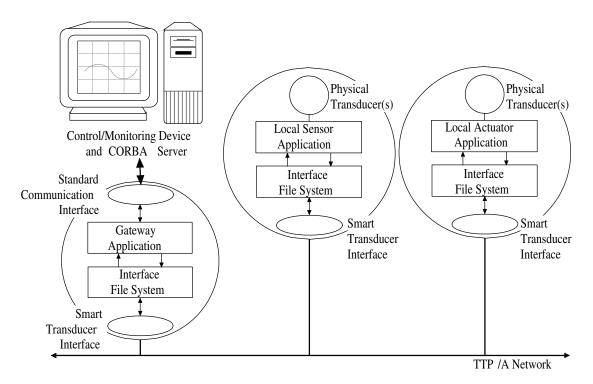
Figure 2: Example network with TTP/A smart transducers
