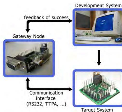
Figure 1: The principle of the automated evaluation
