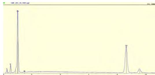
Fig. 5 EDS pattern of ZnO crystal shows Zn is predominated in crystals with aluminium traces (CMF 26 C).
