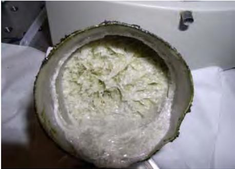
Fig 1 As grown ZnO crystals sitting in Pt-crucible.  $Zn_2B_2O_6$  flux is still sticking on the crystal surfaces. (CMF 8)
