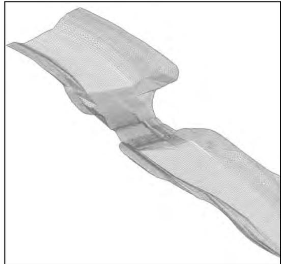
Figure 1: Upstream section of a two-dimensional mathematical model - finite element network
