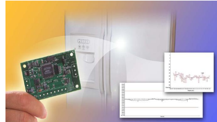
The Grid Friendly™ controller uses data from the power grid to balance energy supply and demand.
