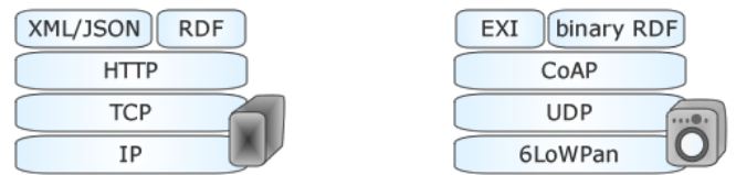
Fig. 2. The HTTP-CoAP mapping: integrating embedded systems in the internet
