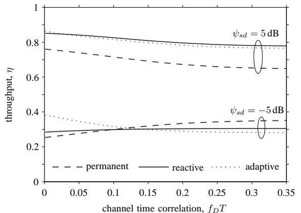
Fig. 6. Throughput  $\eta$  versus channel time correlation:  $f_D T \rightarrow 0$  – quasi-static channels,  $f_D T \approx 0.35$  – i.i.d. channels. Number of potential relays  $N = 5$ , selection overhead  $w = 1$ .
