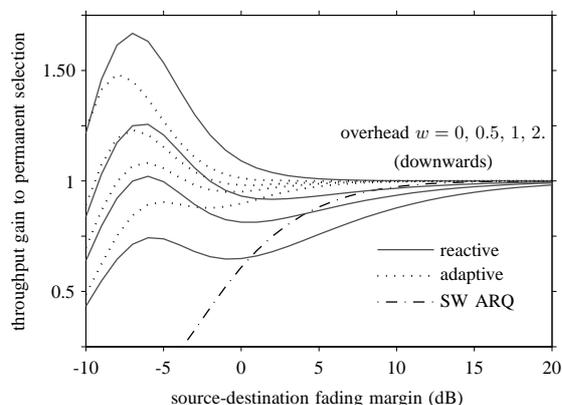
Fig. 5. Throughput gain to permanent relay selection as a function of source-destination fading margin  $\psi_{sd}$  and selection overhead  $w$ . Number of potential relays  $N = 5$ , channel time correlation  $f_D T = 0.1$ .
