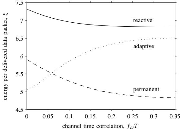
Fig. 9. Expected energy per delivered packet versus channel time correlation:  $f_D T \rightarrow 0$ —quasi-static channels,  $f_D T \approx 0.35$ —i.i.d. channels. Number of potential relays  $N = 5$ ,  $E_{rx} = E_{tx} = 1$ , channel time correlation  $f_D T = 0.1$ ,  $s$ - $d$  fading margin  $\psi_{sd} = -5$  dB.
