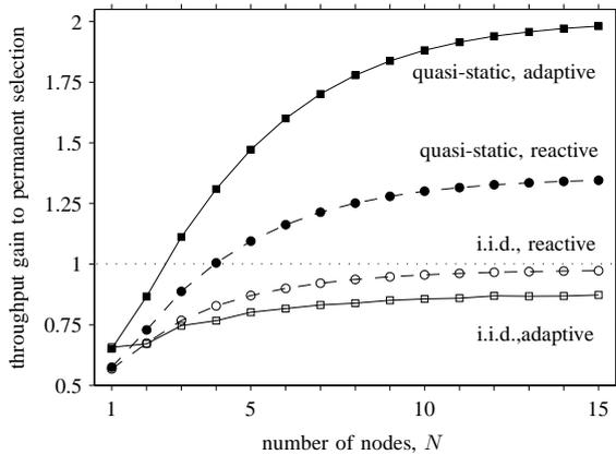
Fig. 7. Throughput gain at correlation boundaries as a function of number of nodes  $N$ . The throughput gain here is the ratio of throughput for reactive/adaptive selection to the corresponding throughput of cooperative ARQ with the permanent relay selection. Selection overhead  $w = 1$ ,  $s$ - $d$  fading margin  $\psi_{sd} = -5$  dB.
