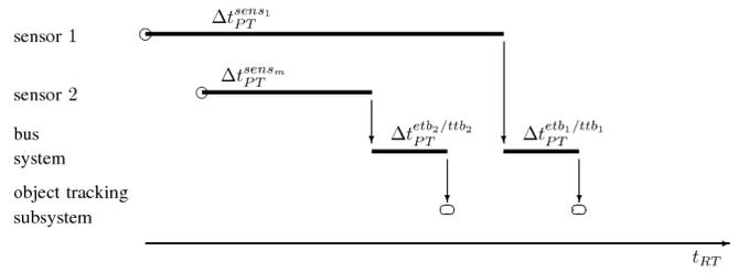
Fig. 1. Out-of-sequence measurement problem
