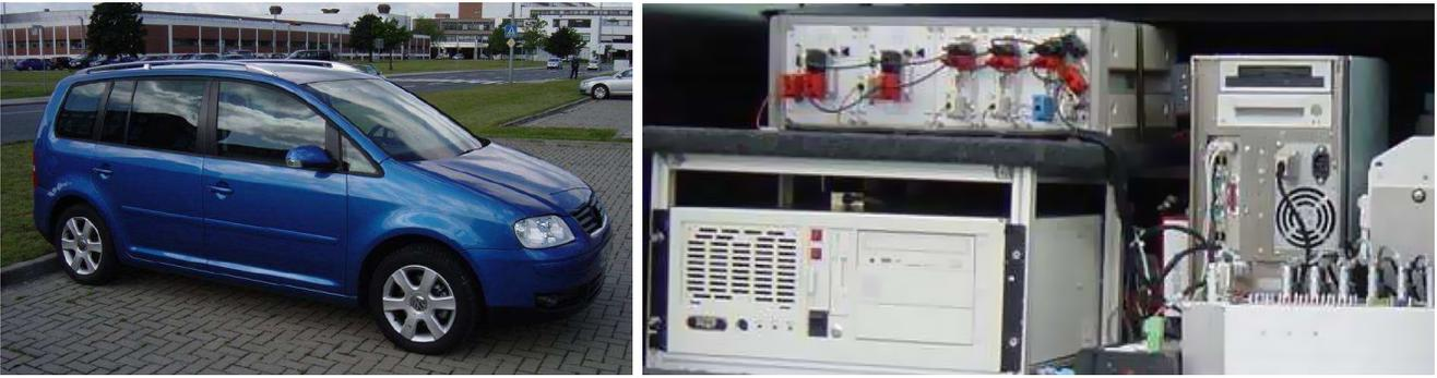
Fig. 3. Test vehicle and hardware installation in the trunk
